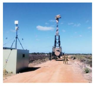
An up-armoured GAMB Radar with Tactical Operations Centre and Waves siren, certifying a CRAM capability at Port Wakefield.
