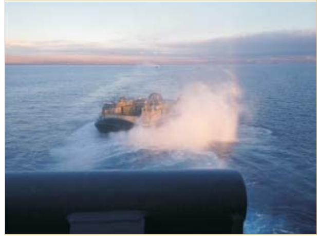
A USMC Landing Craft, Air Cushion (LCAC) returning to the well dock
