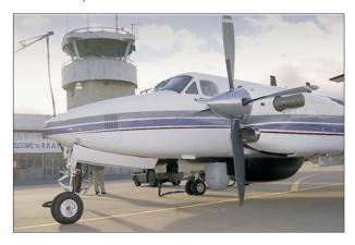
Figure 4: Project Ingara SAR installed on 173 General Support Squadron King Air
